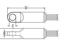
Note: The Rotating Head does not replace the use of a Line Swivel. There are no bearings to allow rotation under load and severe damage may occur to the cable being installed if this product is used without the correct swivel.
