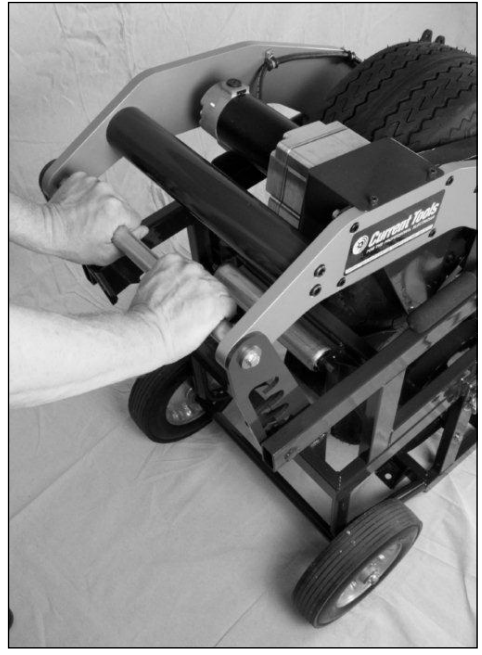
Lifting tension adjustment arms to place resting slots on top of ratchet studs.
