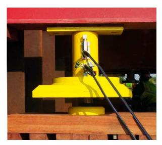
Hydra-Jack™ Climbing Jacks incorporate a hydraulic cylinder inverted inside a specially designed load casing. As the jacks are extended and retracted, block piles are progressively built under the jack for a fast and safe means of raising or lowering large loads or structures.
