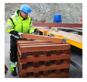
Ideally suited for jacking and blocking applications, Ekki hardwood jacking timbers are exceptionally strong and resistant to crushing and bending.
