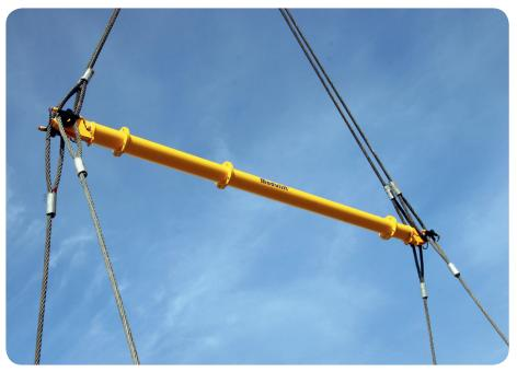
The trunnion spreader is initially available in three sizes up to 1000t capacity.
