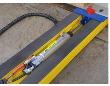
The HT300 features rigid steel tracks capable of carrying loads over unsupported spans, is engineered to push loads up to 300 tons (270 tonnes), and has a working height of only 7" (180 mm).
