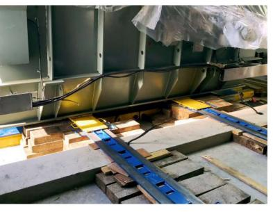
The LP350 is our workhorse low-profile skidding system. Engineered for function and convenience, the LP350 has a durable graphite slide surface and a working height of 1.5" (38mm).
