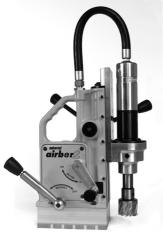
Re-check the unit is correctly positioned for the hole to be cut, and close the magnet handle extension.
