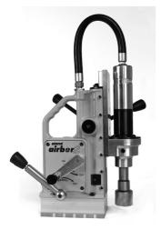
To start the motor, disengage the motor lever locking pin by pulling the handle on motor actuating lever, then move the handle to the left. The motor will start.
