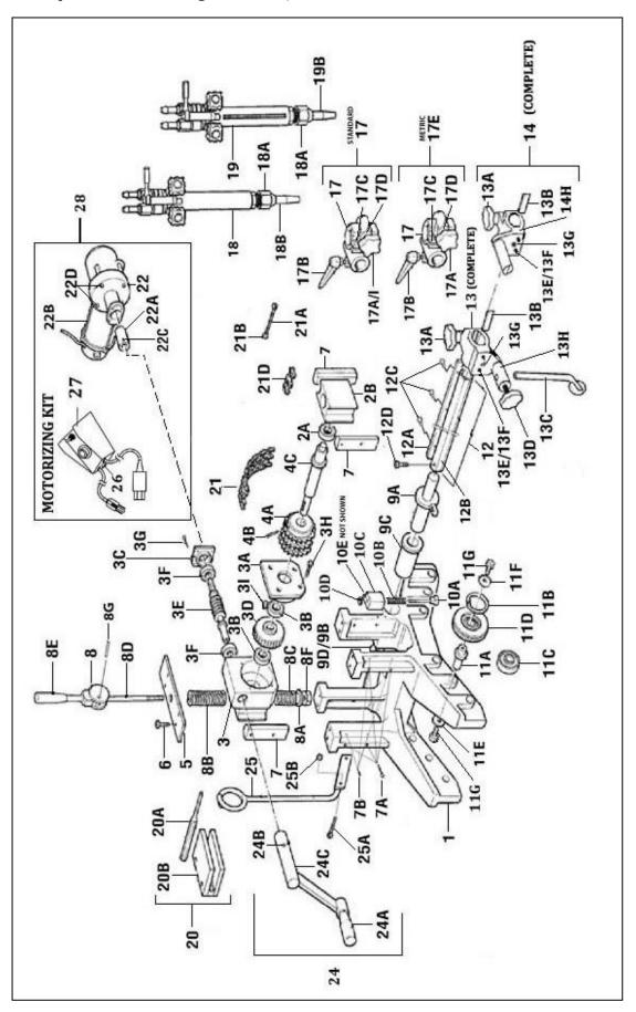
Figure 5 – Exploded Parts Drawing of the Maxi Jolli Chain Machine
