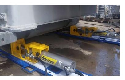
The XLP150 features a 1.25" (32mm) profile, is completely hand-portable, requires limited jacking, and can push or pull up to 150 tons (135 tonnes). It's quote simply one of the most versatile skidding systems we've ever designed.
