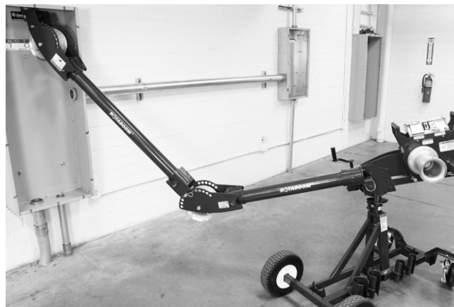
Down Pull using elbow unit and nose unit with RotaBoom™ feature
