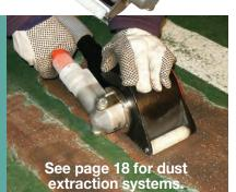
Above: Ergonomic rubber hand grip standard on all new 2" and 4" models. Provides grip for easier pushing along material.
